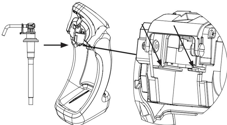
Slide the pump into the guides on the housing and snap the locking tab into place as shown.
