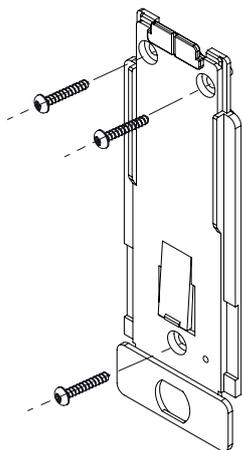
Fasten the wall plate to the wall with the screws and wall plugs provided.
