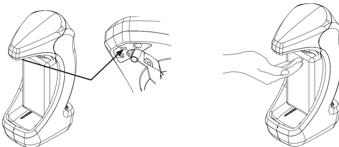
Once the outlet cover is closed, wait 3 seconds for the red LED to go off. To activate the dispenser mechanism, hold your hand under the outlet cover (approx. 5 cm away). This will trigger the dispenser to deliver a stroke.
