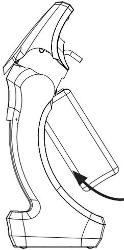
Hold the bottle at a slight angle and slide it over the pump.
