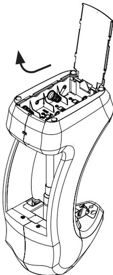
To open the battery compartment, slide the cover towards the back of the dispenser and rotate the cover upwards.
