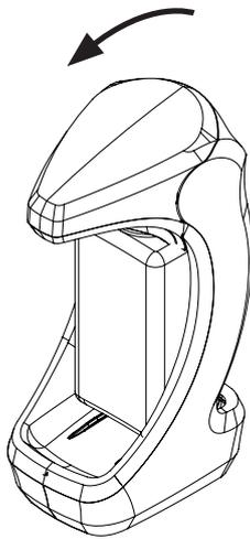
Press down on the outlet cover at the front and make sure that it is closed properly (check the back and sides).
