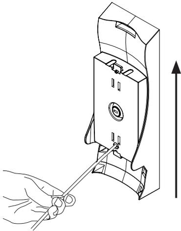
To remove the wall bracket from the wall plate, insert a pointed tool into the hole provided and press the latch of the wall plate backwards. The wall bracket can now be pushed out upwards.
