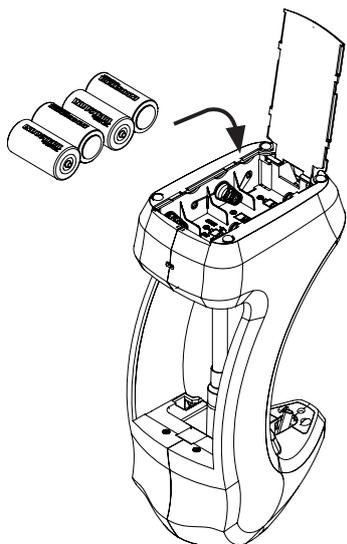
Insert the batteries according to the markings in the battery compartment.
