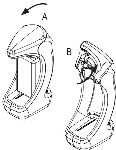
To open the outlet cover, first pull it forwards (A) and then rotate it upwards towards the rear of the dispenser (B).
