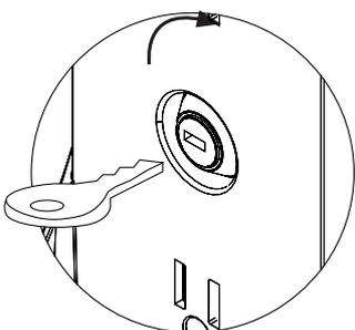
Turn the key to lock the dispenser. Remove the key before inserting the bottle.
