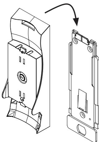
Press the wall bracket against the wall and slide it onto the wall plate until the latch clicks into place.
