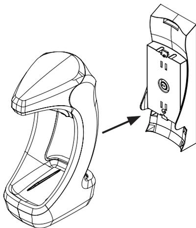
Mount the dispenser on the wall bracket by sliding the opening on the bottle over the rectangular fixture on the wall bracket.
