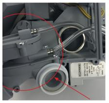
Dismantle sealing cover (3x screws loosen) 3
