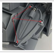
Dismantle sealing part (2x screws loosen)
