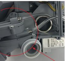
Dismantle sealing cover (3x screws loosen)
